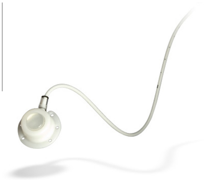
Fig. 1. Plastic bardport low profile. A 10.0 mm height injection plastic (polyoxymethylene) port with a 10.8 mm diameter self-sealing silicon septum is connected to a radio-opaque silicone or polyurethane 6.6 French catheter.
